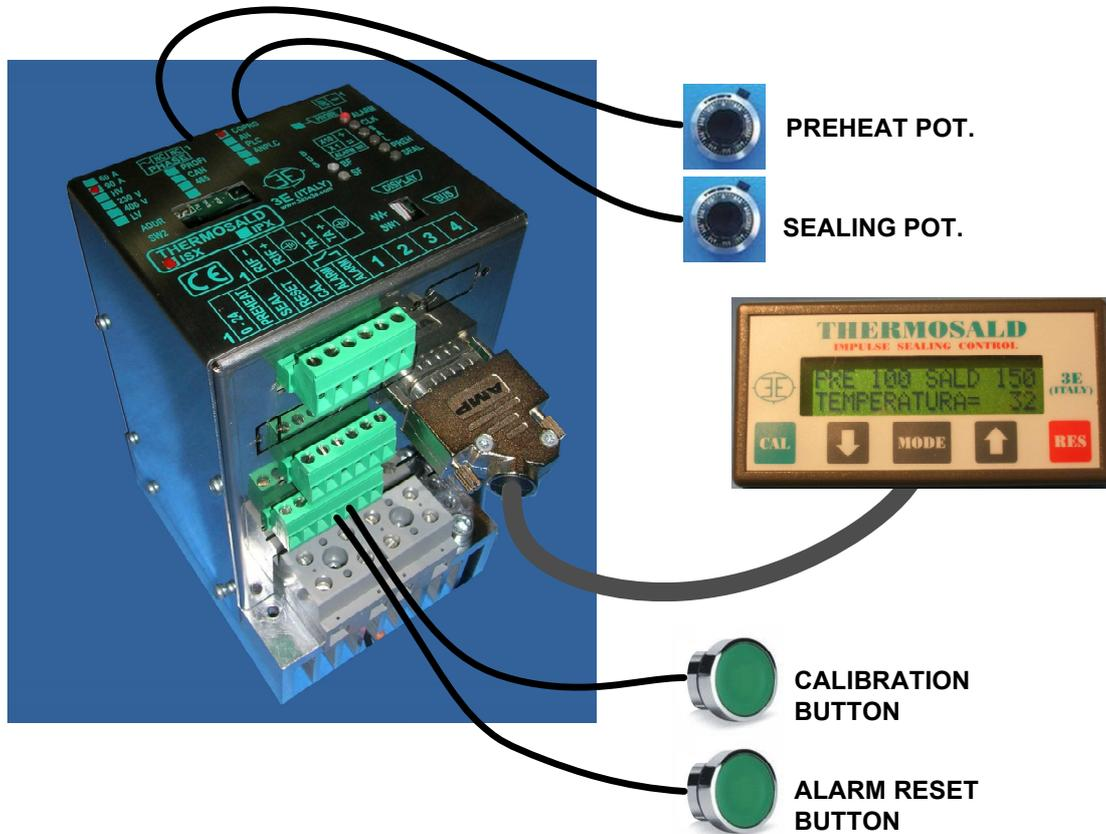
NOTE 1: set the CONFIGURATION MACHINE DATA=1 potentiometers+display to enable the potentiometers.
