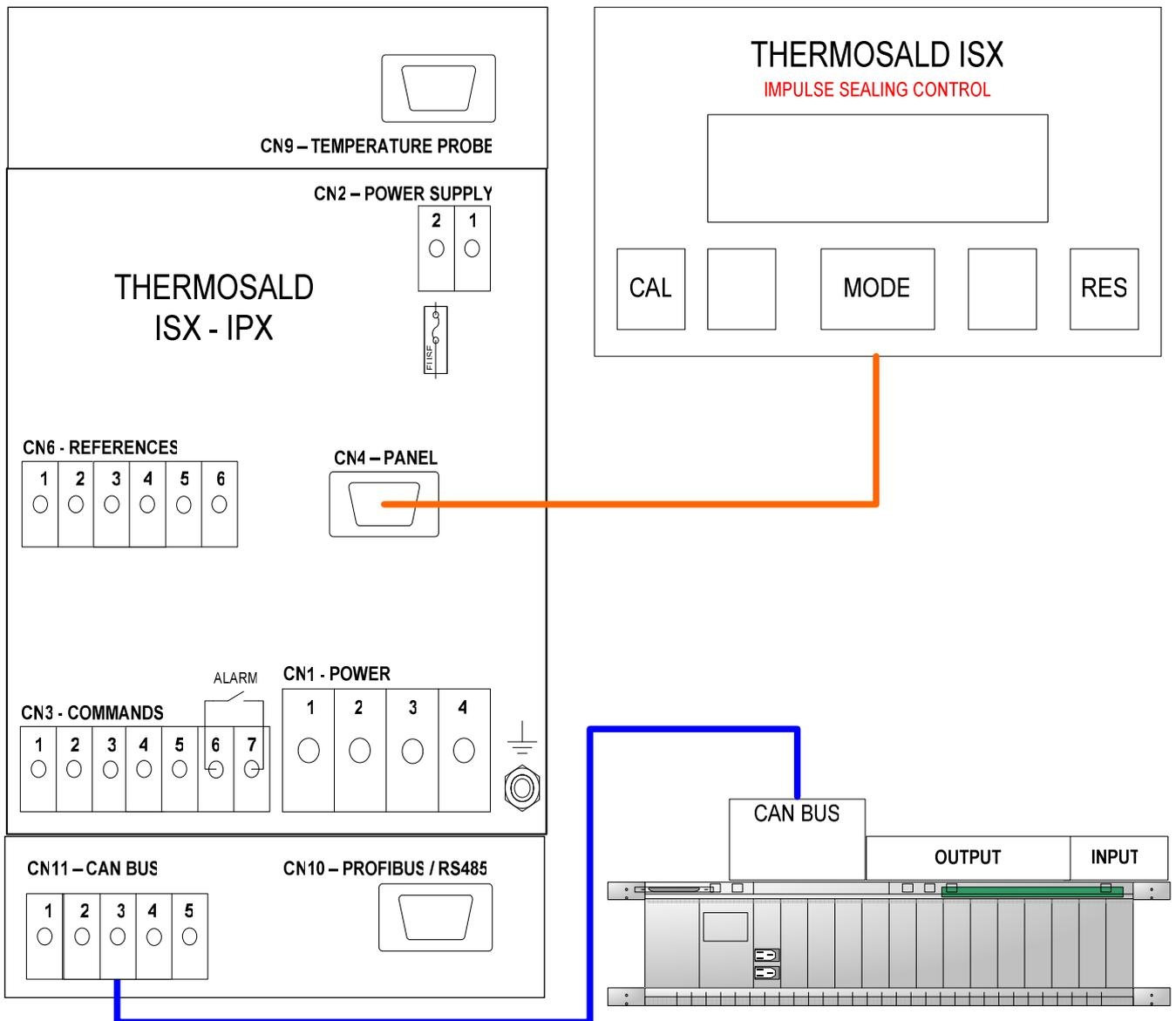
**4.3.8 STANDARD WITH PLC-ANALOGUE OPTION (THERMOSALD ISX2-IPX2 MODEL + OPERATOR PANEL OPTION)**
