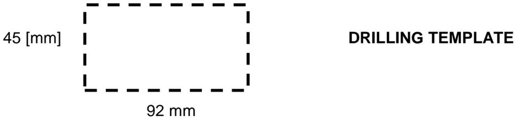
**NOTE: with IP65 protection, code 3ES108Z=IP65, do drilling template 94mm x 47mm,
