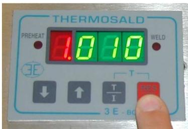
On the display appears “ H100” , to inform that the first heating at 100 degree is in progress; next the writing H200, H100, H200, H100, will appear to inform that cycles of heating and colding at 200 and 100 degrees are in progress. At the end the termoregulator will be ready to work.
