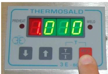
On the display appears “ H100” , to inform that the first heating at 100 degree is in progress; next the writing H200, H100, H200, H100, H200, H100 will appear to inform that cycles of heating and colding at 200 and 100 degrees are in progress. At the end the termoregulator will be ready to work.
