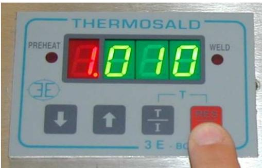
On the display appears “ H100” , to inform that the first heating at 100 degree is in progress; next the writing H200, H100, H200, H100, H200, H100 will appear to inform that cycles of heating and cooling at 200 and 100 degrees are in progress. At the end the thermoregulator will be ready to work.
