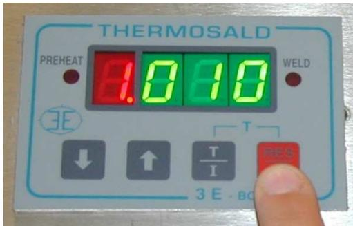
On the display appears “ H100” , to inform that the first heating at 100 degree is in progress; next the writing H160, H100, H160, H100, H160, H100 will appear to inform that cycles of heating and cooling at 160 and 100 degrees are in progress. At the end the thermoregulator will be ready to work.
