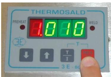
On the display appears “ H100” , to inform that the first heating at 100 degree is in progress; next the writing H200, H100, H200, H100, H200, H100 will appear to inform that cycles of heating and colding at 200 and 100 degrees are in progress. At the end the termoregulator will be ready to work.
